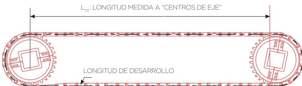
$$Z8(\text{mm}) = 2 \times L_{CE} + 200 \text{ mm}$$
