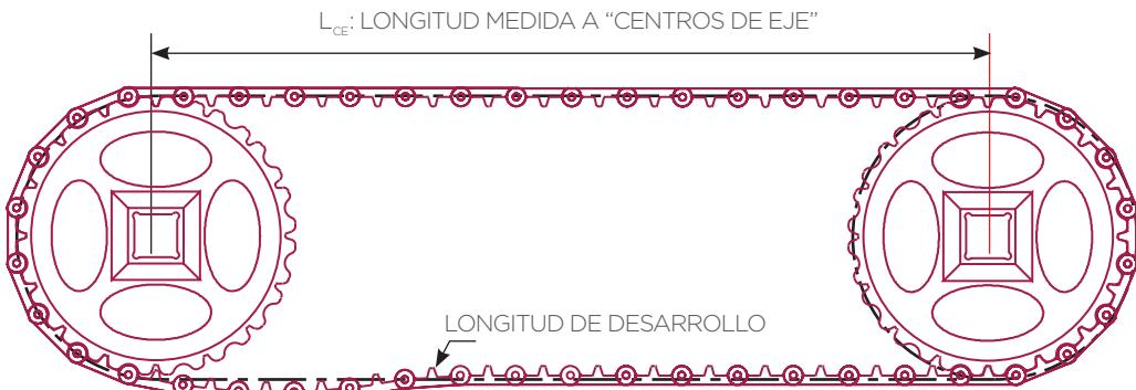
$$Z16(\text{mm}) = 2 \times L_{CE} + 800 \text{ mm}$$
